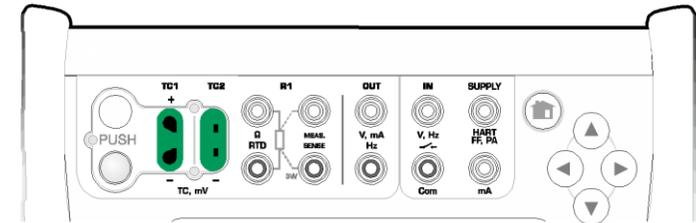
*Thermocouple measurement terminals.
