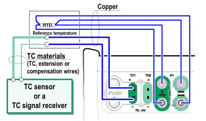
*An RTD connected to R1 terminals measures the Reference Junction temperature.*
