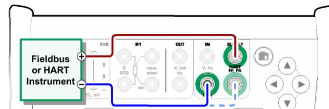
*Digital communication using MC6-Ex's internal power supply.*
