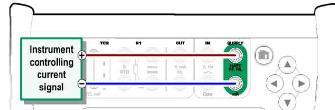
Current measurement terminals. Internal supply
