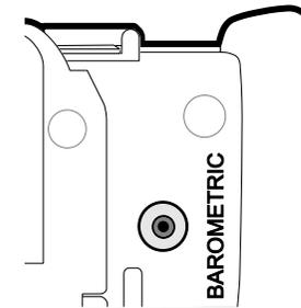
*Venting hole of the Internal Barometric Module.*
