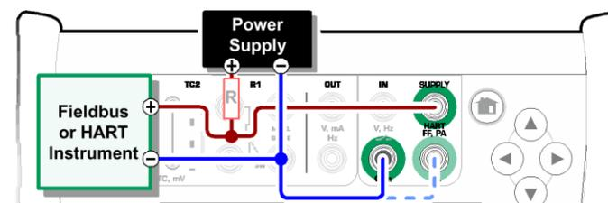
*Digital communication using an external power supply. Include resistor R if power supply is not fieldbus compliant.*
