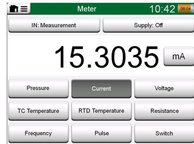
*Current Measurement using Meter*
