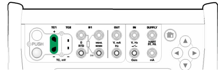
*Thermocouple simulation terminals.
