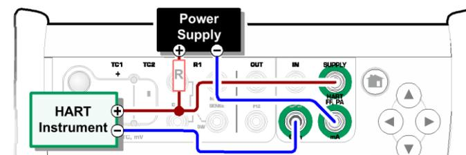
*Simultaneous digital communication and analog measurement with HART Instrument. For connection using internal supply, see page 68.*
